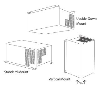
This versatile deck mount converter can be installed in any position, making RV design more flexible for manufacturers. Mount the converter vertically with the fan at the bottom to enhance cooling. WF-9800 Series converter features easy horizontal installation and can even be installed upside down.
