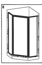
Step 8 A). Apply clear silicone as shown on both the Outside AND Inside of the enclosure wherever aluminum meets Pan / Surround.
