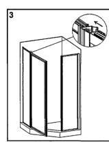
Step 3 A). From the outside of the unit, determine which side the Door will pivot from. B). Slide pivot side of Door frame onto Panel at 180 degrees as shown. Lift Door Frame approximately 1/2" above pan while engaged with panel, then rotate the Door Frame to 135 degree position and set it down onto the top of pan. Door rotation allows Door and Panel to engage and hold together.
