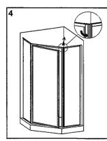
the Door frame with other Panel and push the top of the Door frame and Panel joint toward the back corner of the shower to start engagement of the Door frame to the Panel.
