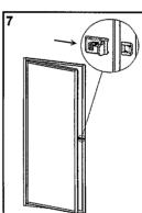
Step 7 From outside of enclosure, open the door and slide travel latch handle onto the pre-installed travel latch base (in the direction from inside of the door toward the outside of the door) as shown.
