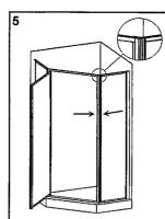
Step 5 A). Compress the 135 degree strike joint from the inside of the shower. Start from the bottom and work upward to engage the entire inside edge. Repeat for the 135 degree pivot joint. B). Ensure good vertical alignment of the Door Frame and Panels. Fasten Door Frame and Panels together through pre drilled holes on the inside of unit about mid height using (1) #8 X 5/8" TEK screw for each joint.
