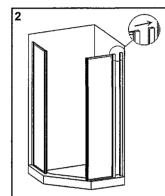
Step 2 A). Identify the Left and Right Panels. The Left Panel has an identification sticker. B). Slide Left and Right Panels onto the Inner Wall Jambs as shown making sure the 135 Degree Post of the Panel faces the inside of the shower. The Left Panel Identification should be on the outside of the shower.
