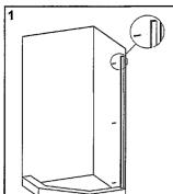
Step 1. Place Inner Wall Jamb against wall and use a level to plumb jamb. Attach using (3) #8 X 1 1/2" SQ PN SM screws. Repeat for other Inner Wall Jamb.
