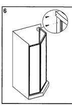
Step 6 A). Place Fascia (i.e. Header) onto top of unit and adjust entire enclosure using available movement in wall jambs until the reveal above the Door is even with the Top Header. B). Attach Fascia to unit with #8 X 5/8" TEK screws through the pre drilled holes as shown.
