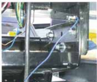
Accelerometers on pin box
