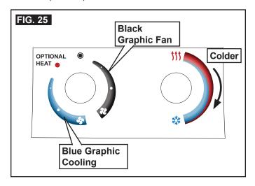
The thermostat controls the compressor On/ OFF operation within a temperature range of approximately 65° F and 90° F measured at the ADB inlet.
