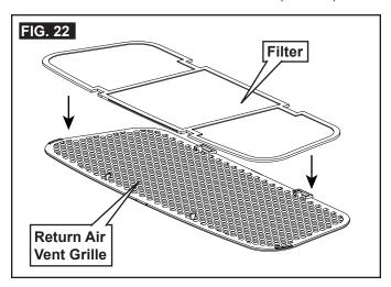
6. Install return air vent grille into the ADB. Slide return air vent grille tab into slot in ADB and rotate up and snap in place. See (FIG. 22).
