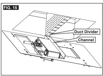
f. Hold the ceiling template up to the roof opening and start each mounting bolt, by hand, through the ceiling template and up into the unit base pan. See (FIG. 16) & (FIG. 17).
